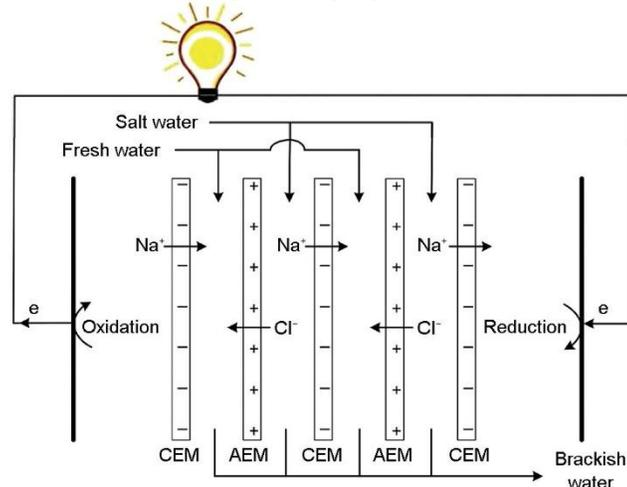
Fig. 1 Principle of reverse electrodialysis (RED)
