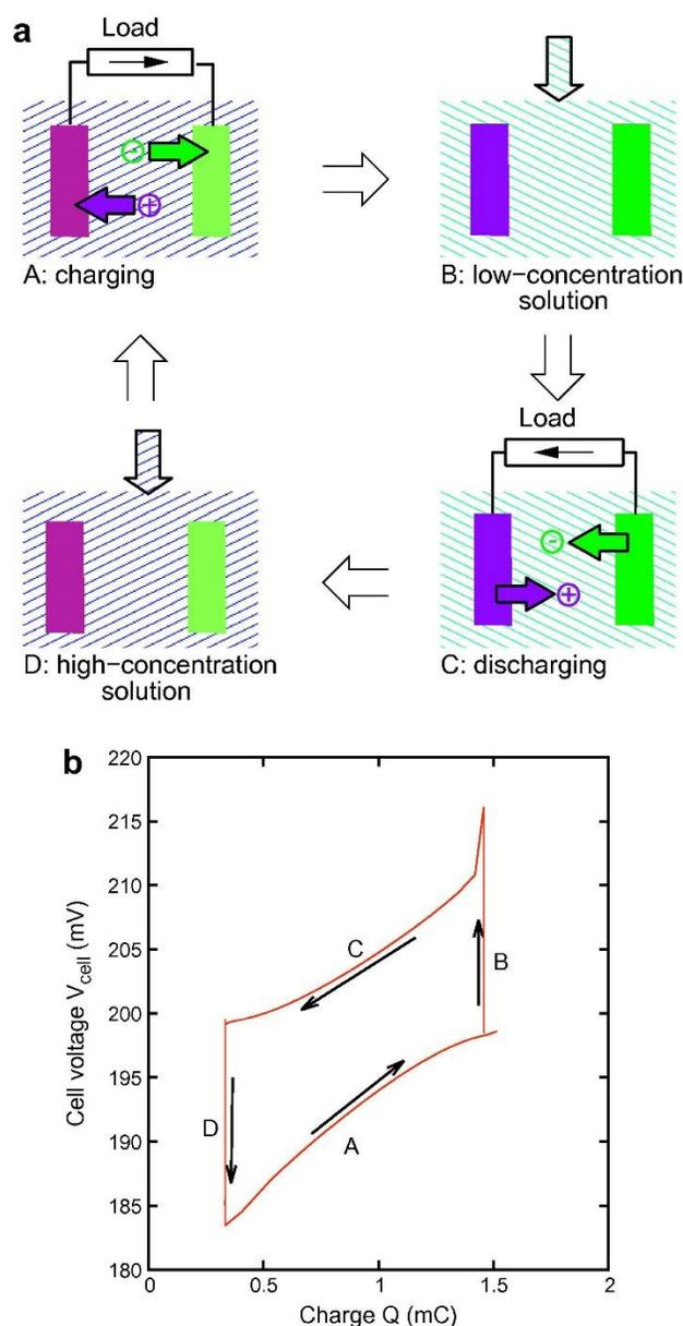
Fig. 2 Principle of capacitive mixing (CAPMIX) – method for energy extraction from salinity gradient. Part a: the cycle characteristic. Part b: the cycle presentation” the voltage versus charge graph. A - charging; B - flow of low-salinity solution; C - discharging; D - flow of high-salinity solution (after [24])
